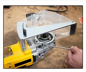
Place Blade Bandit, and bushing if needed, around the snout of the angel grinder and tighten the two screws to secure the shroud to the grinder.
