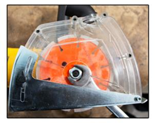
Place standard blade, tuck point blade, or crack chasing blade over shaft adapter and tighten down with shaft adapter nut.
