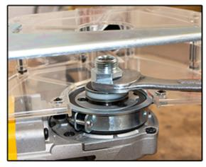
\*When required, screw shaft adapter onto the shaft of the angle grinder.
