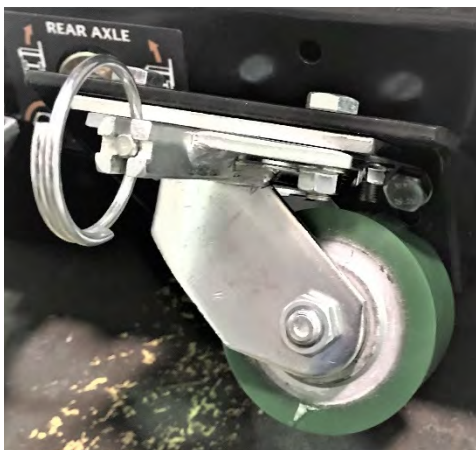
Bogie Wheel – Locked Sideways Position
