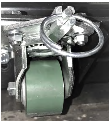
Bogie Wheel – Locked in Free Motion Position
