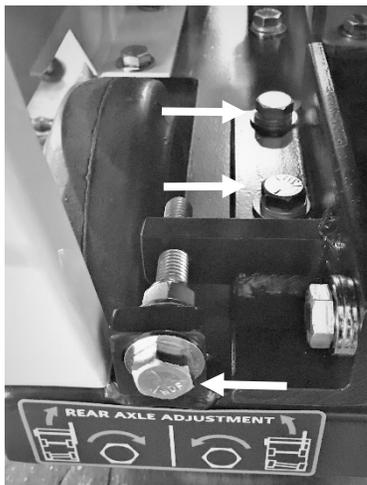
**Rear Axle Bearing Screws and Adjustment Bolt**
