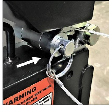
**Detent Pin with Guard Fully Upward**
