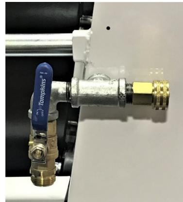
**Water Supply Fitting and Left Water Flow Control Valve**
