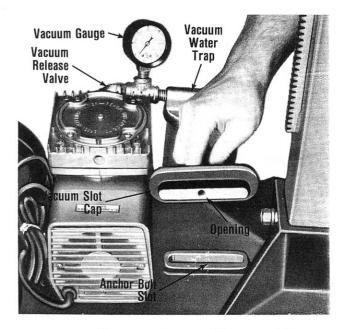
Figure 2. Vacuum Motor and Base.
