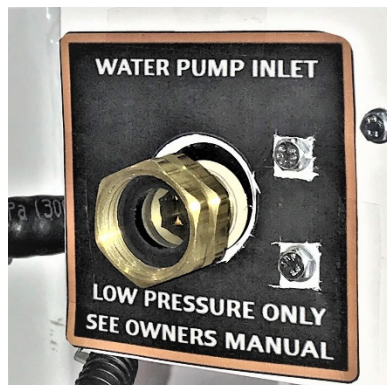
Low Pressure Water Pump Inlet
