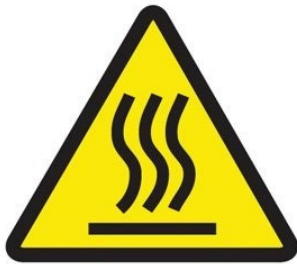
Burn Hazard / Hot Surface
