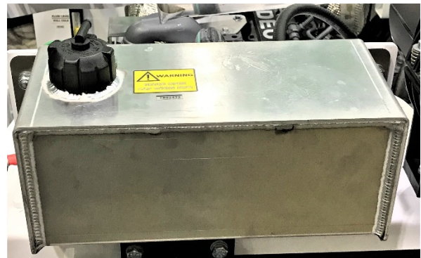
Coolant Expansion Tank
