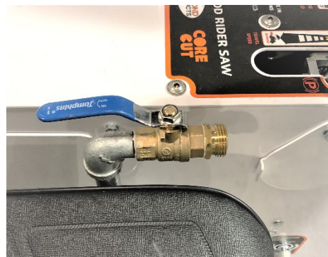
Water Control Valve (ON Position)
