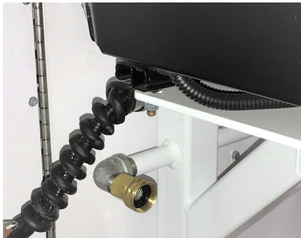
High Pressure Water Hose Connection
