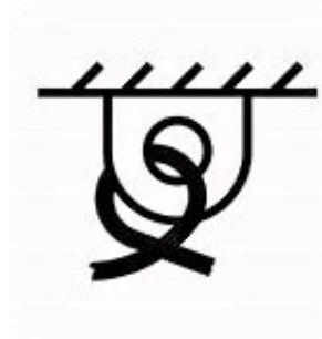
Tie Down Point
