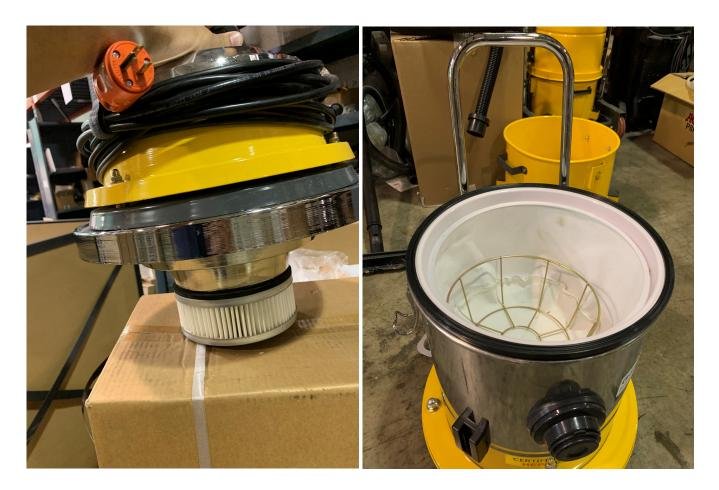
**Note**: The hepa filter, main filter and collection bag are all installed.
