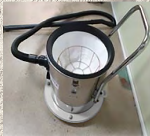
Pre-Filter for Dry Containment
