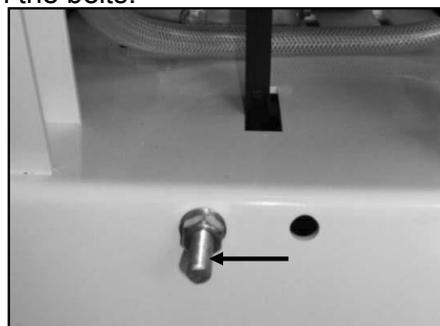
Figure 27: Adjustment Shaft and Nut
