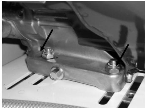
Figure 26: Engine without Adapter Plate/Mounts
