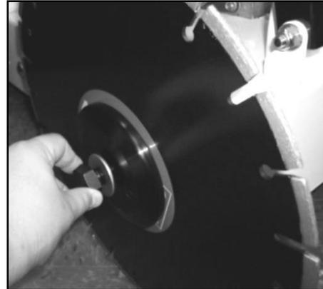
Figure 13: Tightening the Nut
