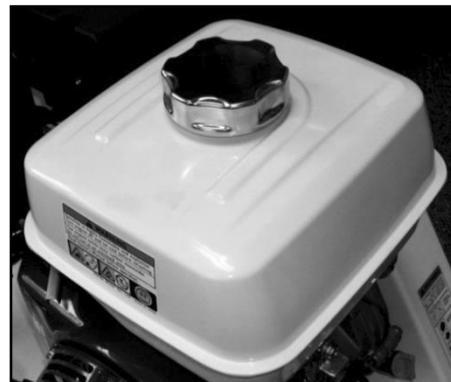
Figure 19: Fuel Tank and Cap
