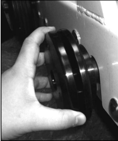
Figure 11: Separating the Flanges
