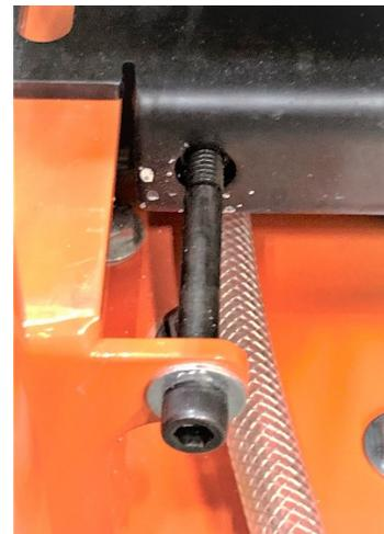
Drive Belt Tensioning Bolt
