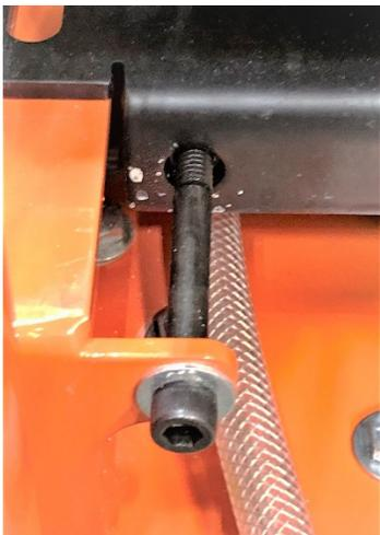
Drive Belt Tensioning Bolt
