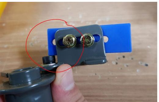
6. If the chip is broke or worn down, replace chip.
