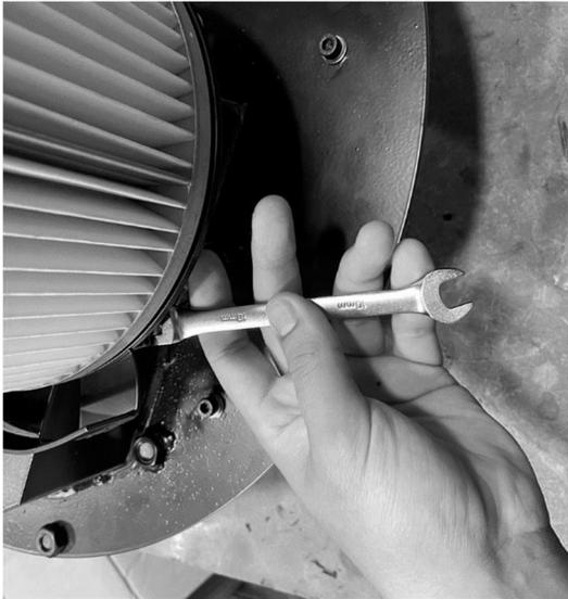
3. Remove the nuts and bolts holding the chip to the bracket
