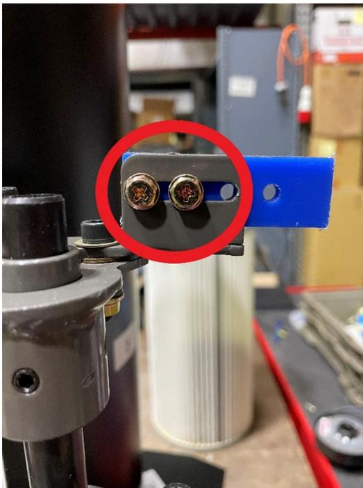
4. If the chip is too aggressive on the filter, slide the chip so that there is less contact.
