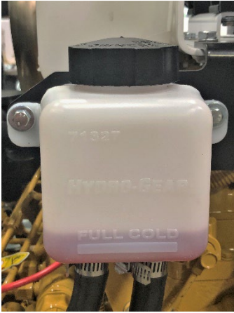
Hydro Pump Reservoir Tank
