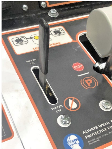
Water Control Valve
