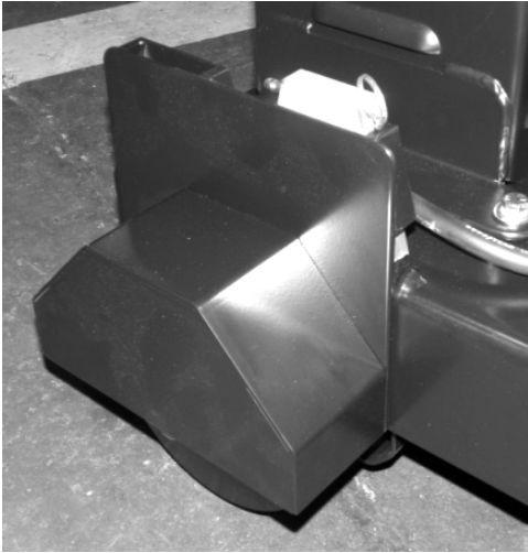
Flange Guard Installed
