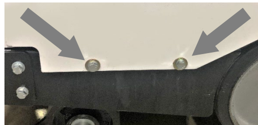
Rear Belt Guard Bolts (Lower)
