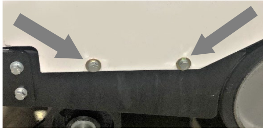
Rear Belt Guard Bolts (Lower)
