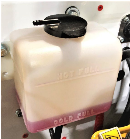
Coolant Recovery Tank
