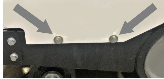
Rear Belt Guard Bolts (Lower)
