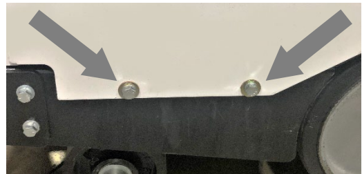
Rear Belt Guard Bolts (Lower)
