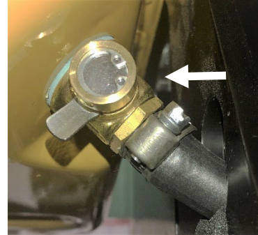
Oil Drain Valve.
