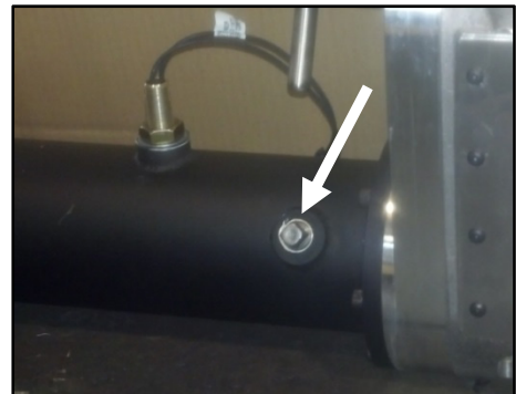
Figure 83: 3/8" Overflow Pipe Plug
