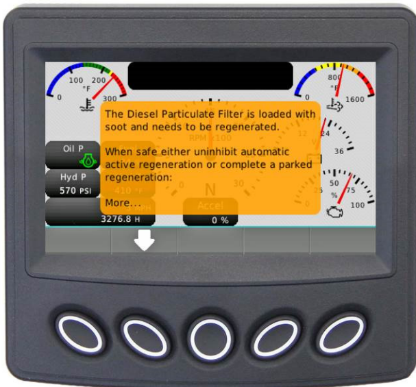
Figure 54 Orange Regen Caution Screen 1 Example of message that requires down soft key.
