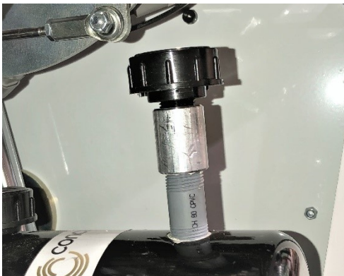
Hydraulic Lift Pump Breather Cap
