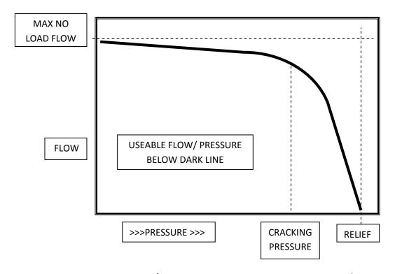
Flow decreases as engine/motor RPM drops under load. Relief valves begin to open and shunt flow to tank at 75-80% of the relief setting (cracking pressure). This further reduces flow to the tool. At relief, all flow is directed to tank.
