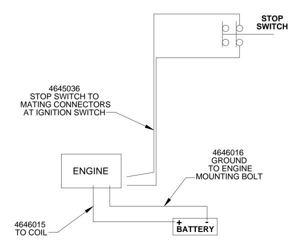
FOR EASE OF ASSEMBLY, ATTACH WIRES TO STOP SWITCH BEFORE INSTALLING IN PANEL.
