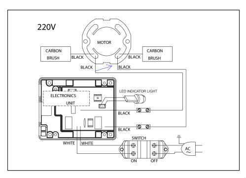
MODEL: CB744 / 4 Speed Diamond Core Drill
