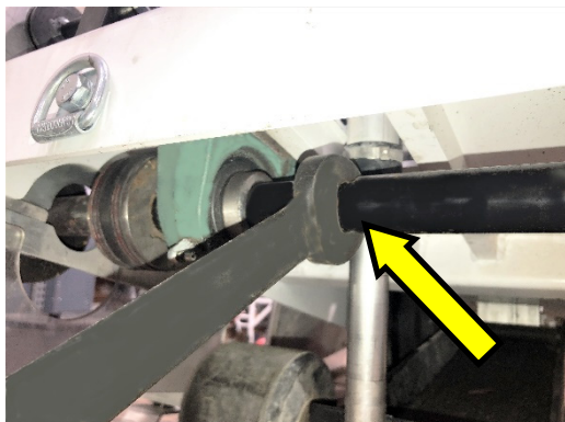
Wrench on Blade Shaft Flats
