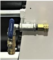
Water Supply Fitting and Left Water Flow Control Valve
