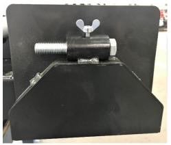
Flange Guard with Blade Shaft Bolt
