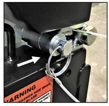
**Detent Pin with Guard Fully Upward**
