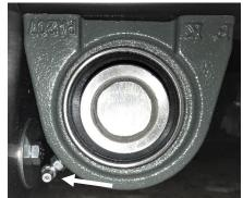
Front Axle Bearing Grease Fitting
