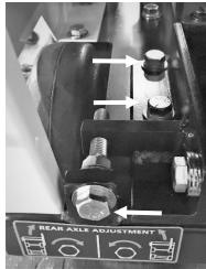
Rear Axle Bearing Screws and Adjustment Bolt
