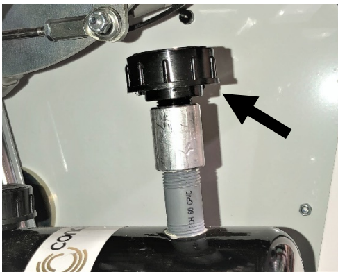
Hydraulic Lift Pump Breather Cap
