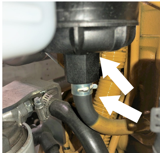
Clip and Hose Connected to Lower Cap
