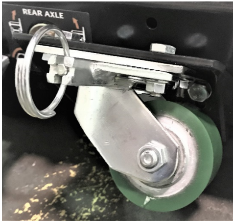
Bogie Wheel – Locked Sideways Position
