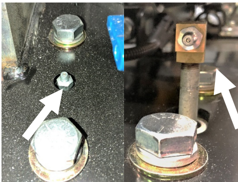
Grease Fittings – Blade Shaft Bearings
