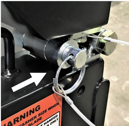
Detent Pin (26" Blade Guards and Larger)
