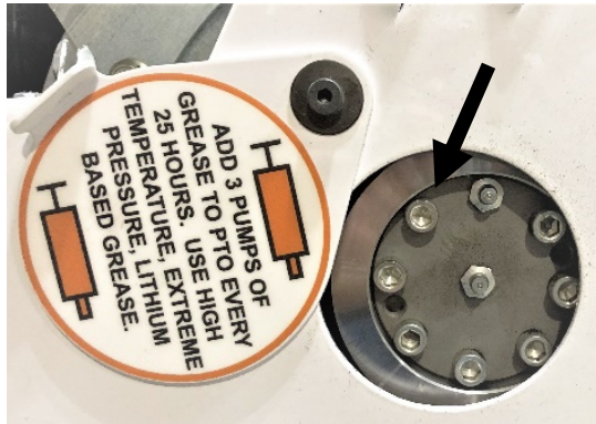
PTO Grease Fitting
