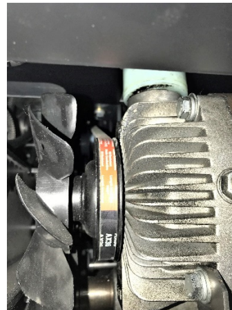
Secondary Transmission Belt
