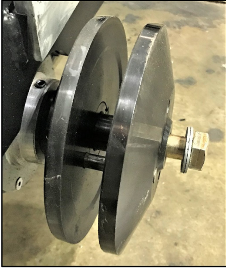
Blade Flanges Separated
