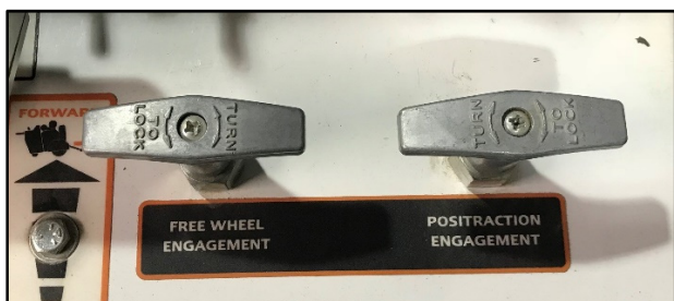
Free Wheel and Positraction Engagement
