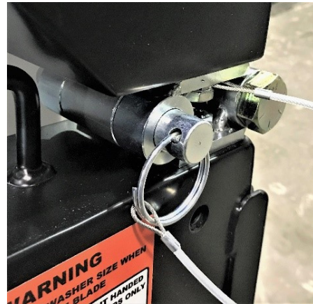
Detent Pin (26" Blade Guard and Larger)
