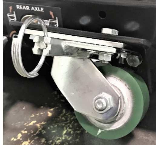
Bogie Wheel – Locked in Sideways Position
