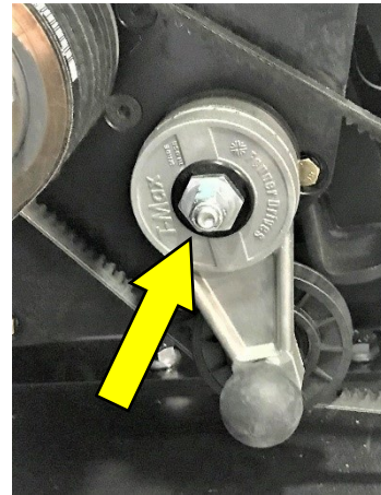
Rotary Tensioner, Body Nut & Mounting Nut
