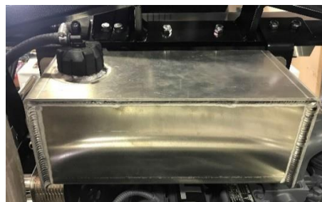
Coolant Expansion Tank
