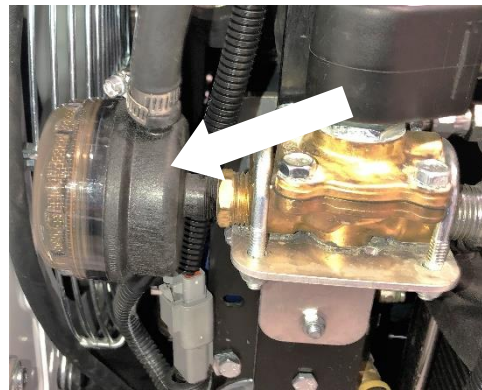
Water Inlet Strainer
