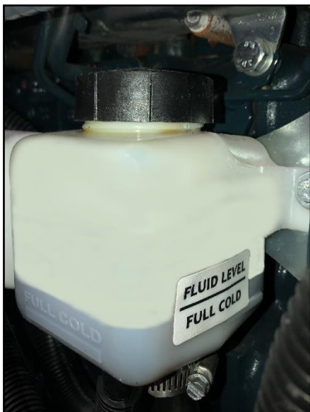
Hydro Pump Reservoir Tank
