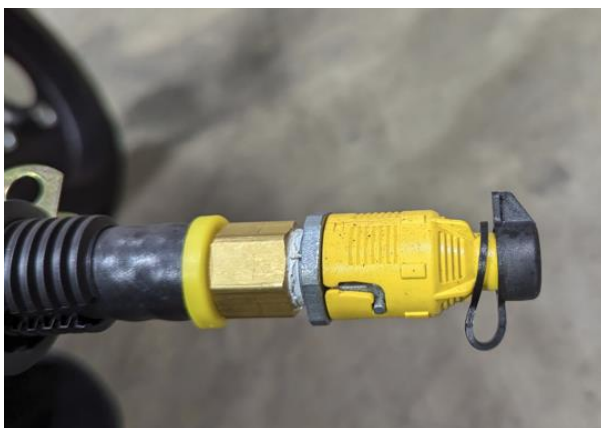
Oil Drain Valve
