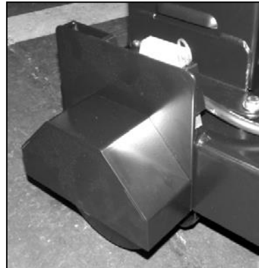
Flange Guard Installed
