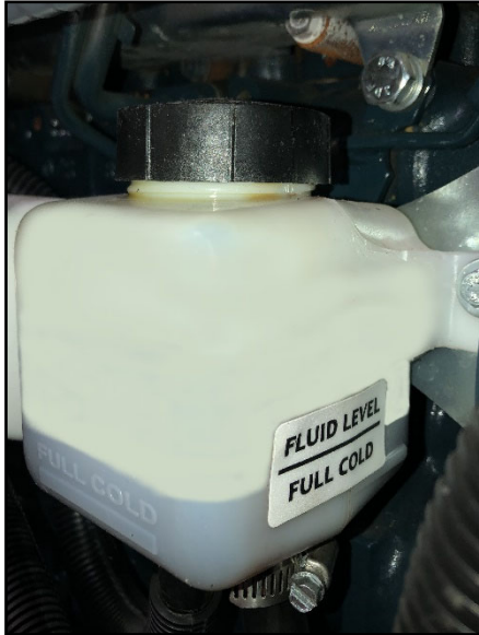
Hydro Pump Reservoir Tank
