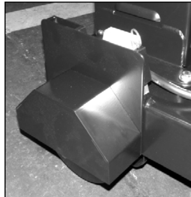
Flange Guard Installed
