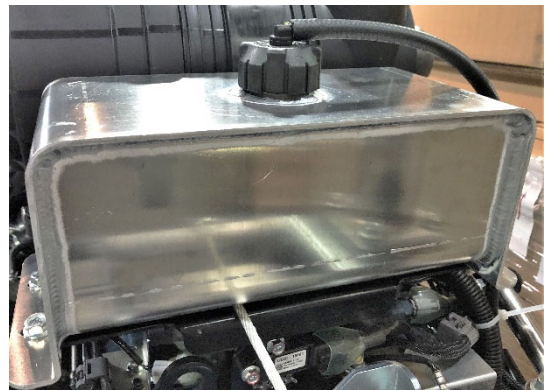
Coolant Expansion Tank
