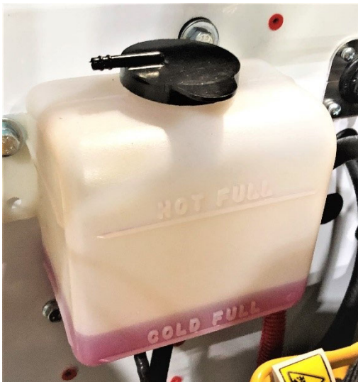
Coolant Recovery Tank
