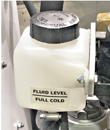
Hydro Pump Reservoir Tank
