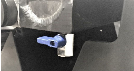
Radiator Drain Valve
