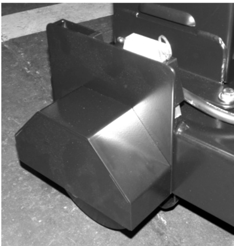
Flange Guard Installed
