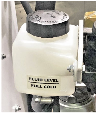
Hydro Pump Reservoir Tank
