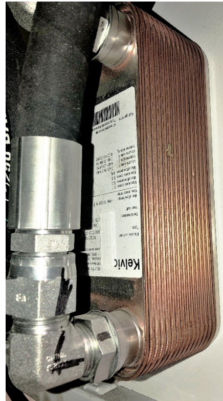
Hydraulic Oil Cooler
