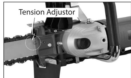
2. While holding the guide bar upward from the nose end, turn the tension adjuster clockwise to tighten.
