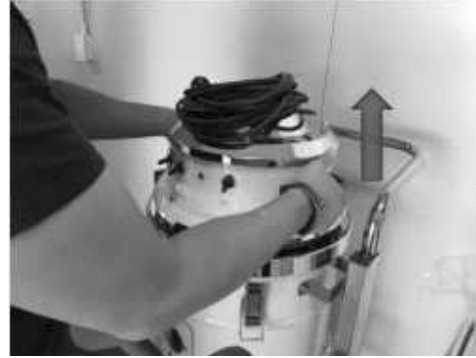
2. lift the head of a vacuum cleaner
