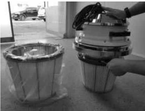
3. prepare the motor for replacement.
