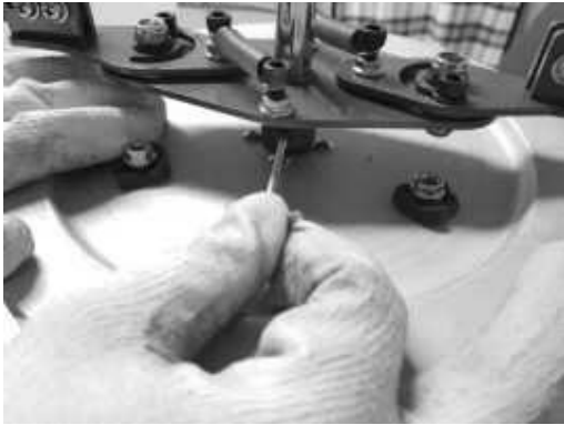
7. Remove hepa filter
