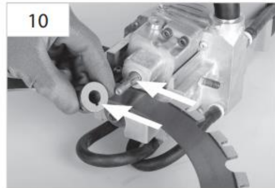
10 Mount the smooth driver roller; when doing so, observe the key and keyway.
