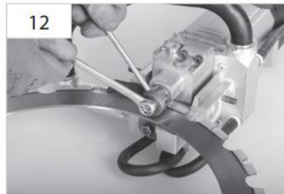
12 Tighten the smooth drive roller. Tool: 1/2" spanner and a punch
