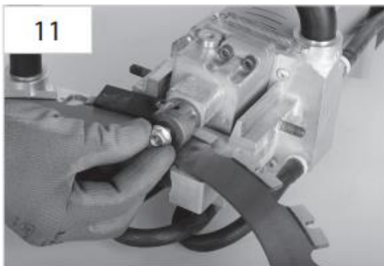
11 Screw on the smooth driver roller by hand.
