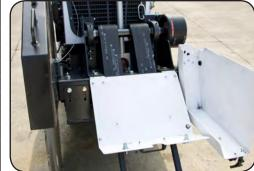
**Easily Accessible Belts**Multi-panel openings for quick belt maintenance.
