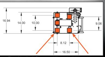
Five wide wheels for saw stability and reliable tracking
